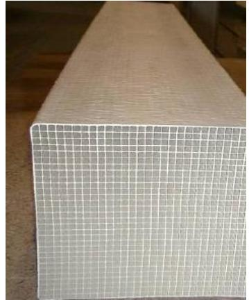
The catalyst: ceramic - based on titanium
