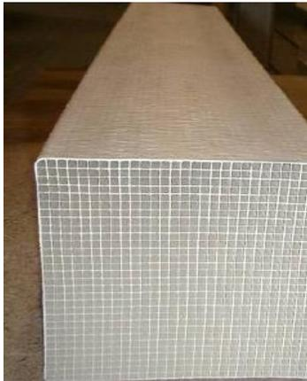
The catalyst: ceramic - based on titanium
