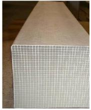
The catalyst: ceramic - based on titanium
